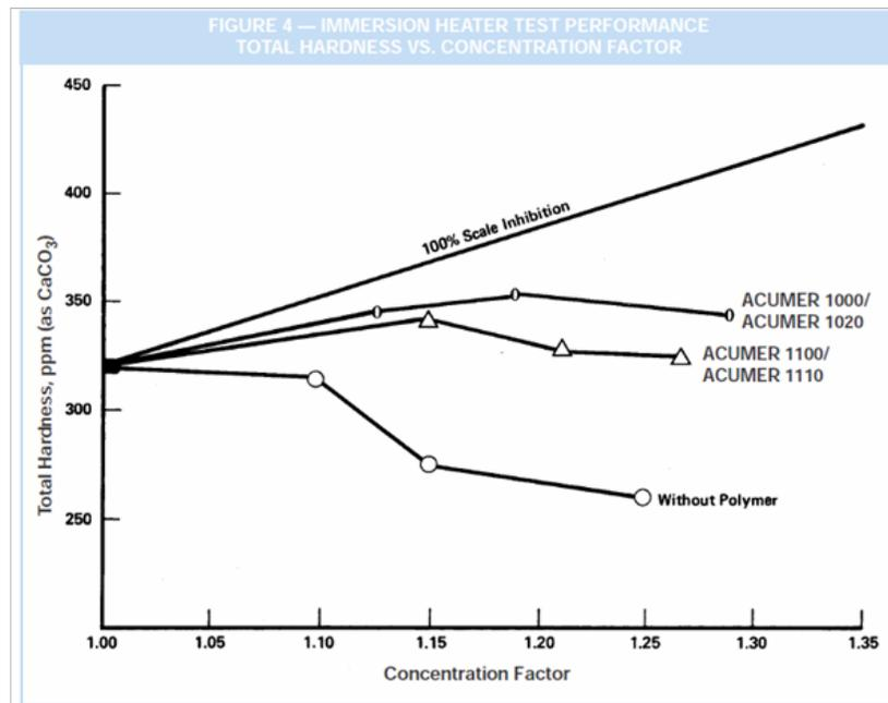
Scale Inhibition at Heat Transfer Surfaces (Con't.)
