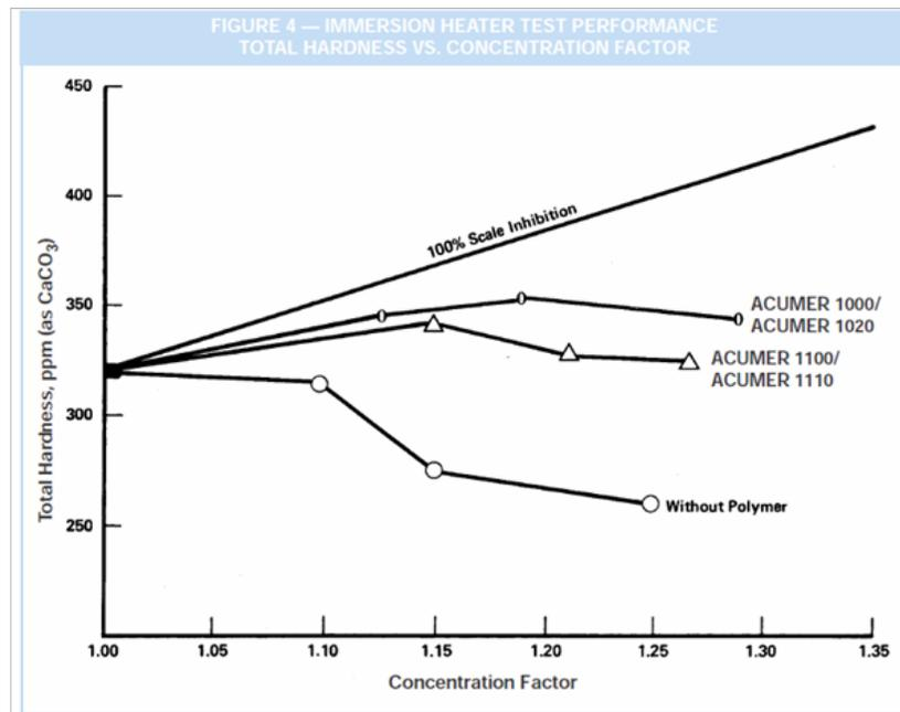
Scale Inhibition at Heat Transfer Surfaces (Con't.)
